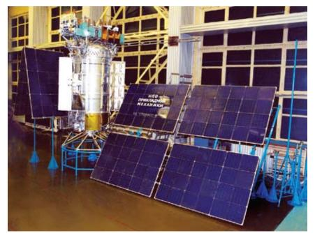
$\label{eq:loss} Increased pointing accuracy of solar arrays will help improve the GLONASS dynamic model.$
