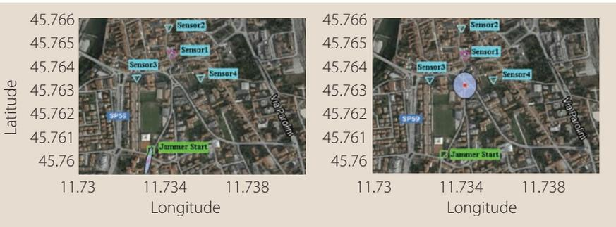
**FIGURE 8** Estimated position using the peaks associated with the spoofing signal (left) and the peaks associated with the authentic signal (right)
